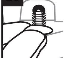
Install a small Christmas tree fastener (D) provided through the hole where you removed the fastener in step 6 and through the existing hole in tab Z of the liner.
